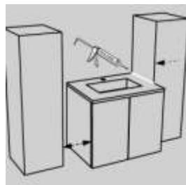
Leave space between the pedestal and the unit under the basin to avoid any water retention zone.
