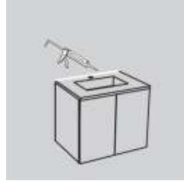
Make sure you put in a water seal between the furniture unit and the wall
