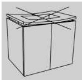
Before installing your counter top, check that it is not warped.
